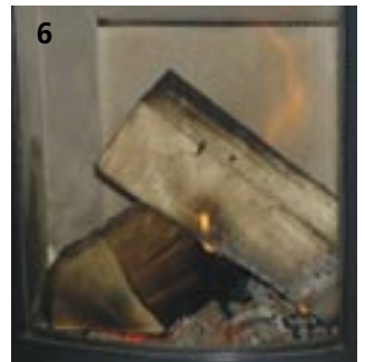
6 Now you can use ordinary firewood. Close the door completely and fully open the combustion air supply.
